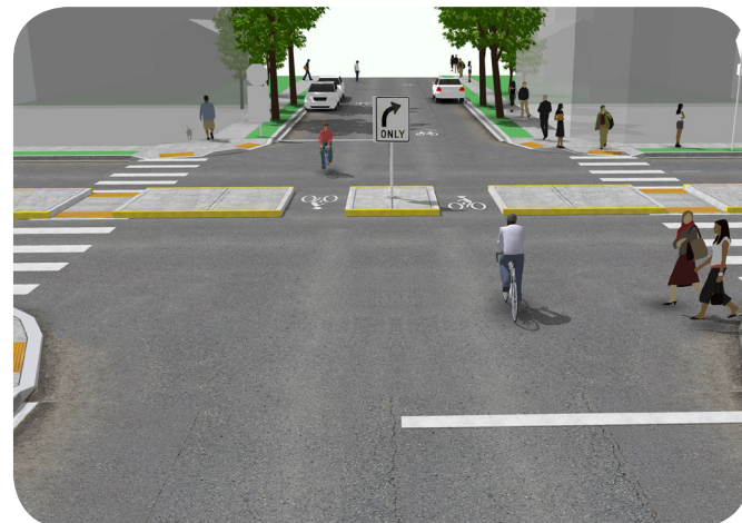
An example of an intersection with bike islands and automobile traffic being diverted. (Source: NACTO)
