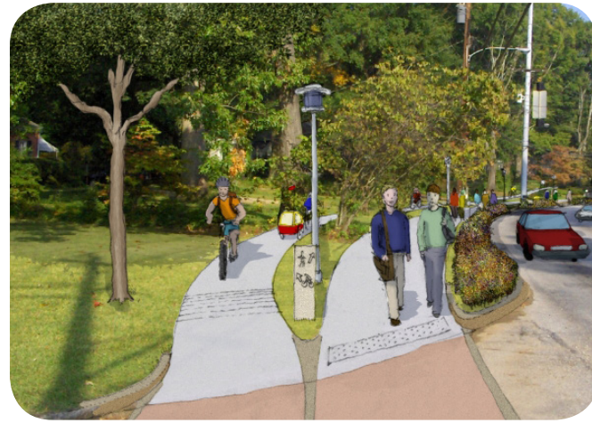
Separated 5-foot paths at intersection with delineated pavement and ADA accessibility (Source: Bike.Emory.edu)
