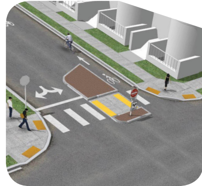
Pedestrian safety island that allows for through bikes, but diverts car traffic (Source: NACTO)
